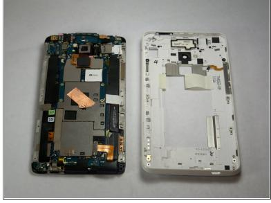
Use the small plastic opening tool to pry between the screen and the rear case.
