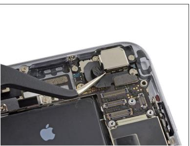
Remove any tape covering the upper left rear-facing camera screw.
