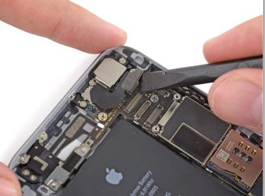
Use the flat end of a spudger to lift the rear-facing camera connector up off of its socket on the logic board.
