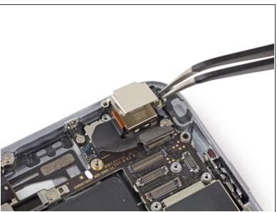
Remove the rear-facing camera bracket.
