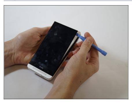
Wedge the plastic opening tool into the crack around the screen on the top, left and right sides.
