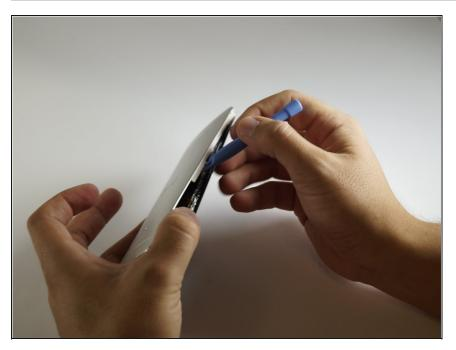
• The rear case is held on by glue and eight tabs on the screen bezel. On the volume side there is one above the rocker and three below; on the SIM side all are below the slot. Insert the plastic opening tool between the case edge and the screen bezel, aiming to prise the rear case edge outwards to loosen the glue and free the tabs, one at a time.
