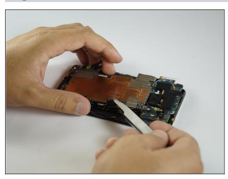
Lift the motherboard completely out of the phone with the <u>tweezers</u>. (may stay attached at the bottom by tape)
