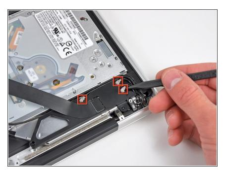
Use the tip of a spudger to pry all three AirPort/Bluetooth antenna connectors up off the AirPort/Bluetooth board.
