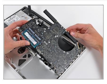
Carefully lift the logic board assembly from the left side and work it out of the upper case, minding the
