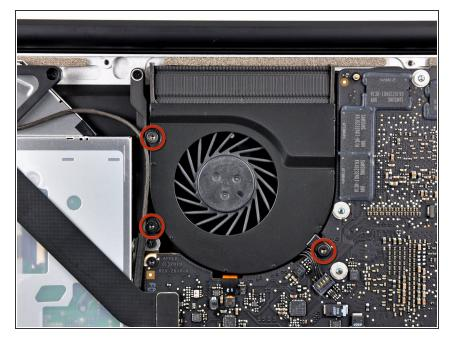
Remove the three T6 Torx screws securing the right fan to the upper case.
