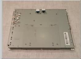
Grasp, lift, and remove the LCD Module from the front panel.
