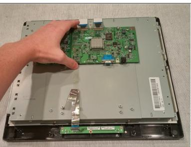
Lift up and remove the joined Power Supply Board and Video Display boards.
