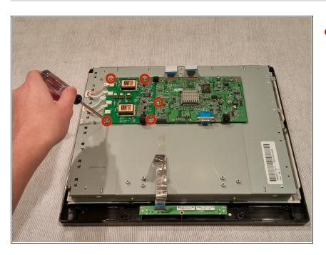
Unscrew the 5 screws holding the Power Supply Board and Video Display boards on.
