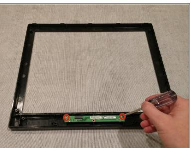
Unscrew the 2 screws holding the Power Button Circuit Board.
