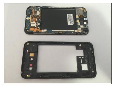
• The inner cover is now removed, you now have access to the many parts on the inside of the phone.
