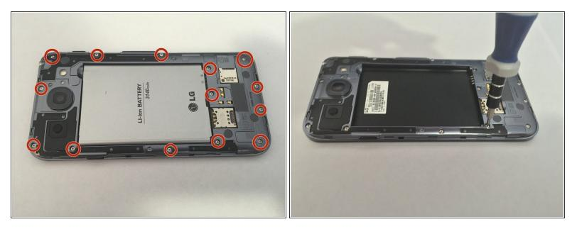
Make sure you remove the battery first. You will see that there are 14 screws on the back of the inner case. Use the Phillips head screwdriver to remove each of the screws, make sure to put the screws in a safe place where they will not get lost.
