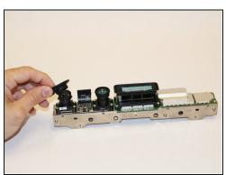
• Go ahead and start by removing the Colour Camera's lens cap. This way you can remove the Camera without anything in your way.
