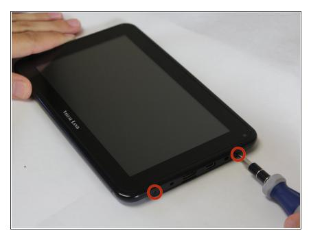
Unscrew the two 4.0mm Phillips head screws found near the ports at the bottom of the device using a PH #00 screwdriver.
