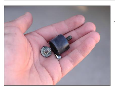
While on the subject, here is one of the other buffers (in this case, the front most). It was a cheap URO brand buffer. The metal part separated from the rubber. I believe it was this that put extra stress on the rear portion of the bracket leading to the fracture. Keeping your rubber buffers in good shape should prolong the life of the bracket.
