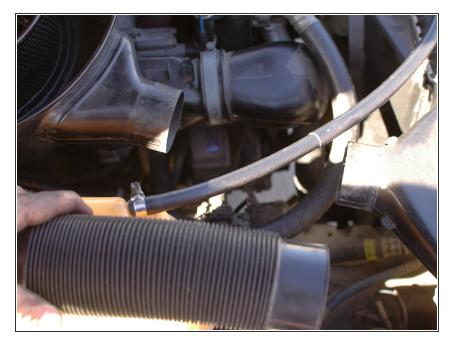
Remove the flexible hose that is between the air cleaner housing and the air intake nozzle above the passenger/right side headlight. It will contract enough to pull off.
