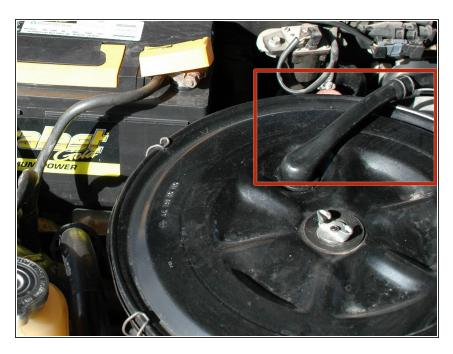
To access the air cleaner bracket the housing must be removed. In order to remove the housing the cover must come off. To remove the cover, start by pulling off the breather hose. It will just pull off.
