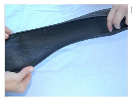
Examine the inside of the tire to check for holes or tears before replacing.
