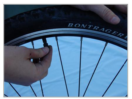
To deflate the tire, remove the cap and attach the pump head to the valve. You should then hear air flowing out from the tire.
