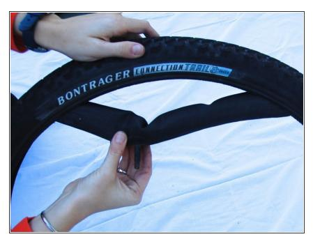
Holding the valve, pull the tube out from the inside of the tire.
