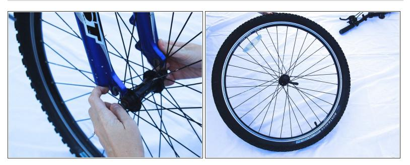
Pull the frame of the bike upwards to separate the front wheel.
