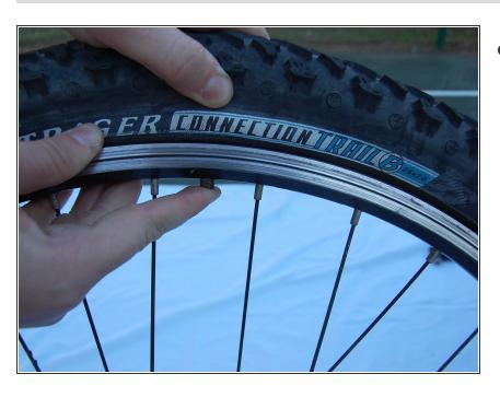
Push the valve upward through the hole in the rim.
