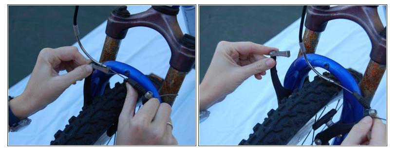
Unhook the brake wire in the metal tube from the brake wire holder on the brake caliper in your left hand.
