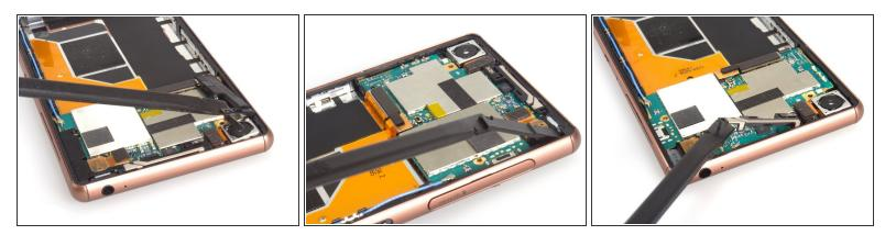
Remove three pieces of securing bracket.
