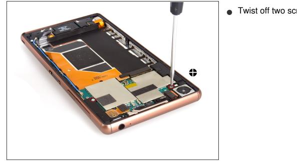
Twist off two screws at first.
