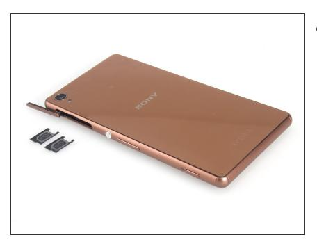
Power off and remove two SIM card trays at first before earpiece speaker replacement.
