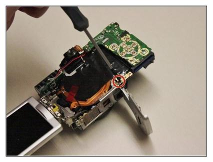
• Remover .2 mm screw using a #00 Philips screwdriver.
