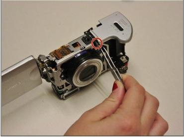
• Using tweezers, gently pull remove the small rod in the battery door hinge.
