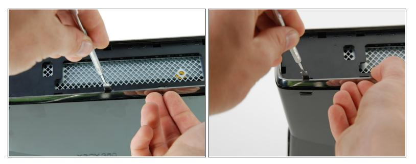
Using the same method described above, free the two remaining clips along the left edge of the top bezel.
