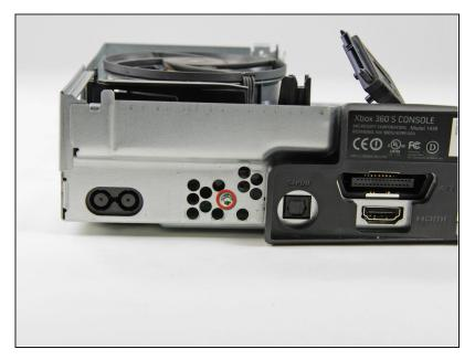
Remove the 11.3 mm T10 Torx screw holding the hard drive bracket to the metal frame, near the DC-In port.
