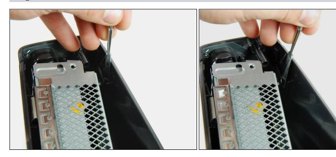
• Release one clip in the front left corner of the top edge securing the left case to the faceplate.
