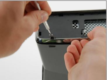
Using the same method described above, free the two remaining clips along the left edge of the top bezel.
