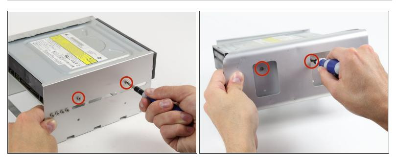
Unscrew the shown two 6-32 type screws on each side of the optical drive.
