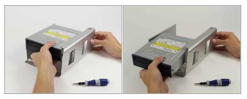
Firmly grasp the optical drive and pull it out of its enclosure.
