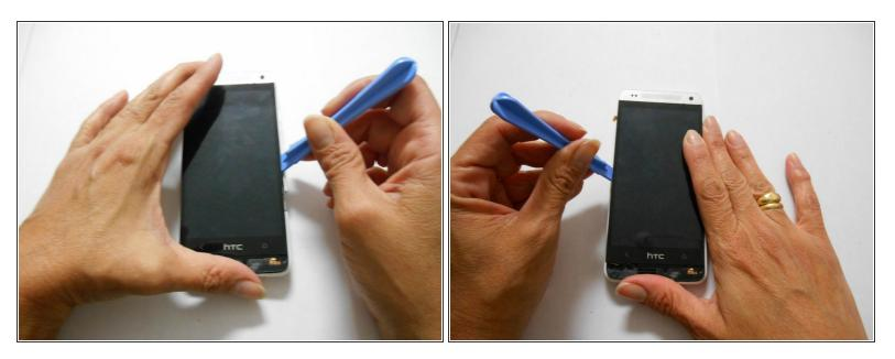
• Using the plastic opening tool, pry on the screen to separate it from the adhesive holding it.
