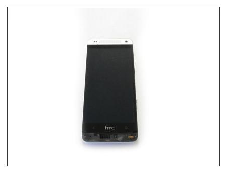
• Use the blue plastic opening tool to pry and remove the bottom speaker grill.
