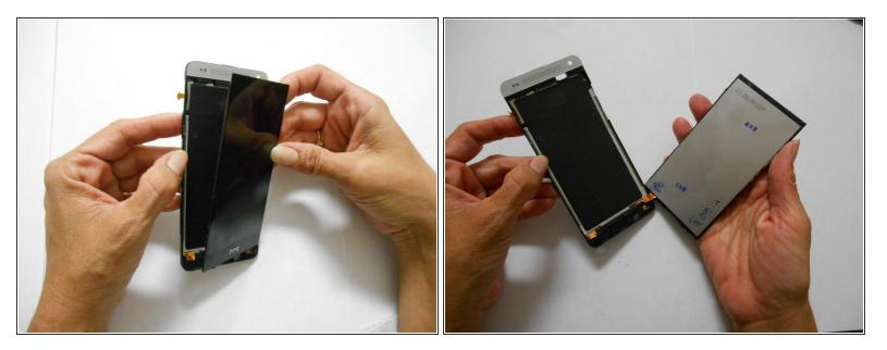
• After you have used the opening tool to pry, use some force to separate the LCD screen from the glue.
