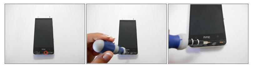
Remove the screw under speaker grill using a T6 Torx screwdriver.
