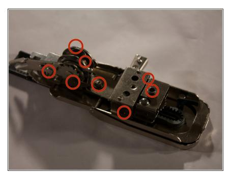
Apply a drop of lubricant at each of the points indicated here.
