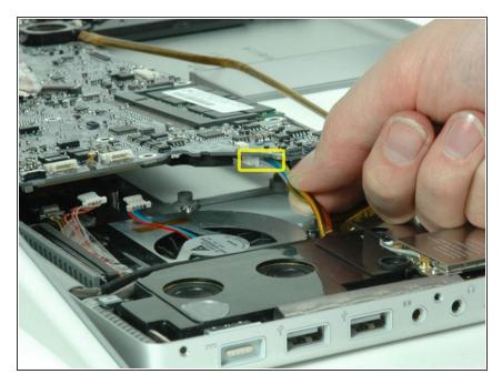
Lift up the left side of the logic board and disconnect the multi-colored power connector from the bottom of the board.
