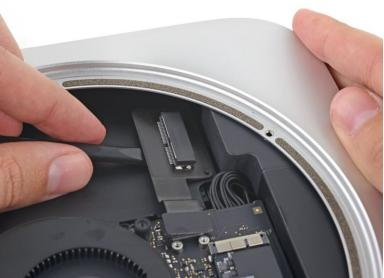
Slip the flat end of a spudger under the SSD cable to lift it off the adhesive holding it to the Macmini.
