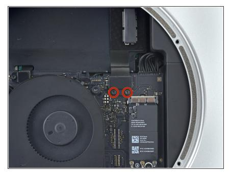
Remove the two 2.6 mm T6 screws securing the PCIe SSD cable bracket.
