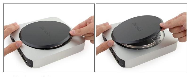
Lift and remove the bottom cover.
