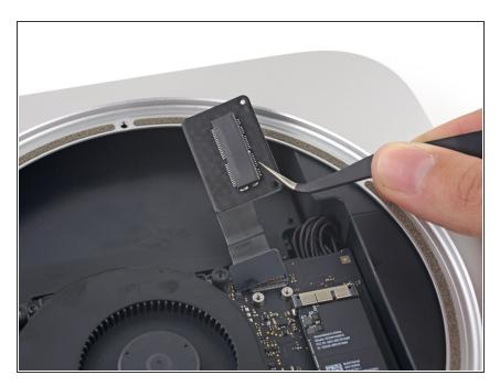
Remove the PCle SSD cable from the Mac mini.
