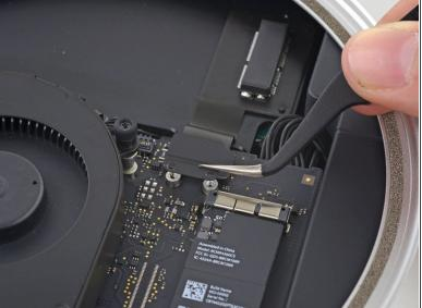
Remove the PCIe SSD cable bracket.
