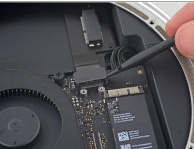
Use the flat end of a spudger to lift the PCIe SSD connector straight up off of its connector on the logic board.
