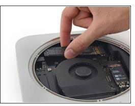
Lift the free end of the SSD up slightly and pull it out of its socket.
