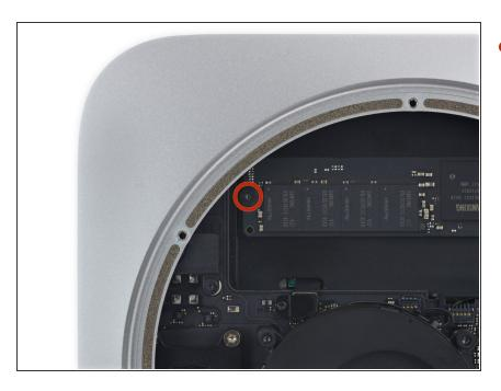
Remove the 5 mm T5 screw securing the SSD.
