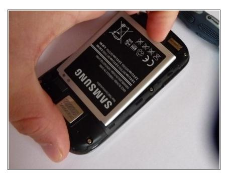
Remove the battery from the device.
