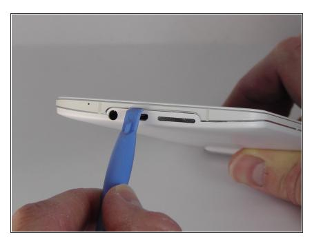
Insert the plastic opening tool into the crevice. The back cover is most easily opened by starting at this location.
