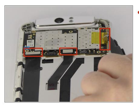
• Use tweezers or fingers to remove the three connector tabs.
