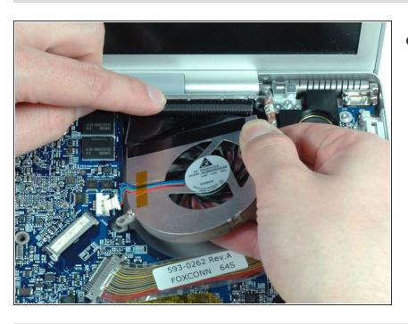
Lift the right fan and its metal bracket out of the logic board.
