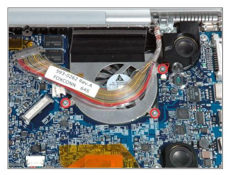
Remove the three silver T6 Torx screws securing the right fan.
