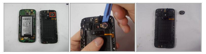
Use the plastic opening tool to remove the Speaker from the protective cover.
