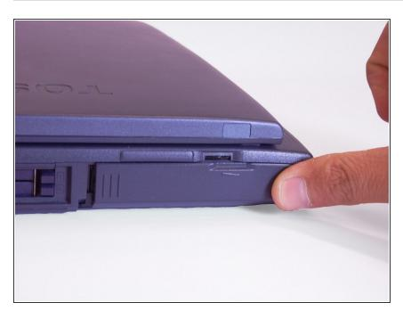
Placing your finger on the raised grip, push the battery casing to the right. It will slide over.
