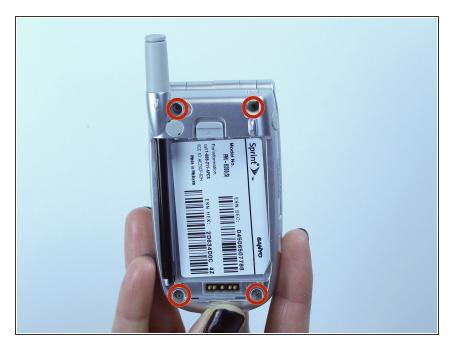
Unscrew all four, 5mm Tri-Wing screws.
