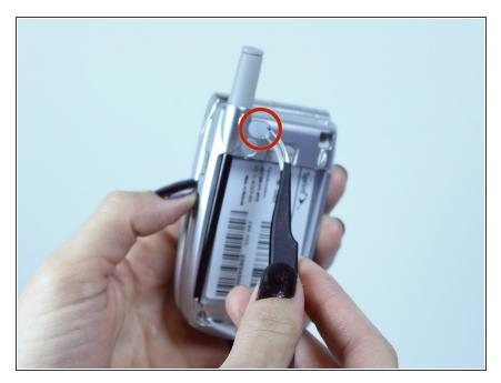
Use a push pin or tweezers to remove the neoprene screw-cover located on the upper, left corner of the back casing.
