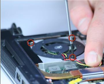
Use a Phillips #0 to remove the three screws holding the fan in place.
