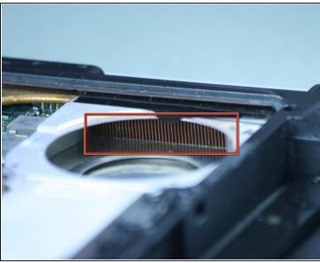
• Use a cotton swab or compressed air to blow air from the inside, out to clear dust from the vent or heat sink.
