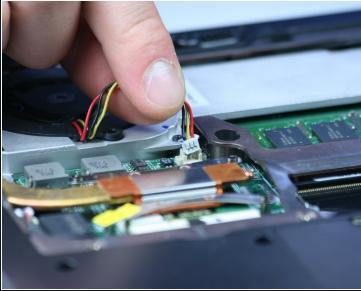
• Unplug the wires by pulling straight up on the white connector and away from the computer.
