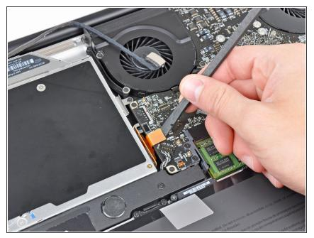
• Use the flat end of a spudger to pry the optical drive connector up and out of its socket on the logic board.
