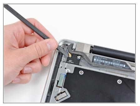
Use the flat end of a spudger to pry the Bluetooth antenna connector up and off its socket on the Bluetooth board.
