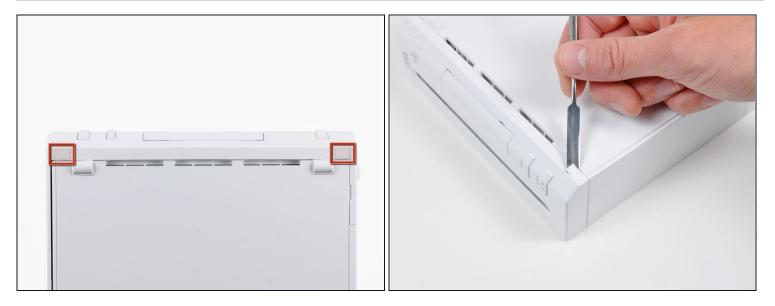
• Use a metal spudger to remove the white plastic screw covers stuck to the lower case near the front of the Wii.
