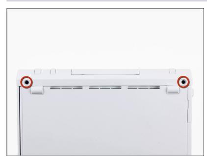
• Remove the two 8.3 mm Tri-Wing screws hidden under the covers you just removed.
