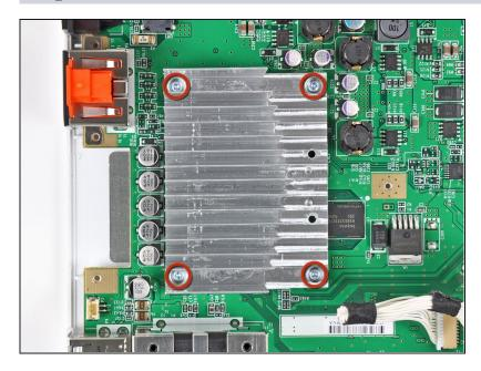
• Remove the four 11.3 mm Phillips screws securing the heat sink to the bottom panel.
