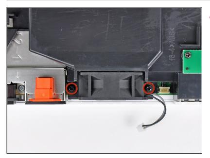
• Remove the two 10 mm Phillips screws securing the fan to the fan shroud.
