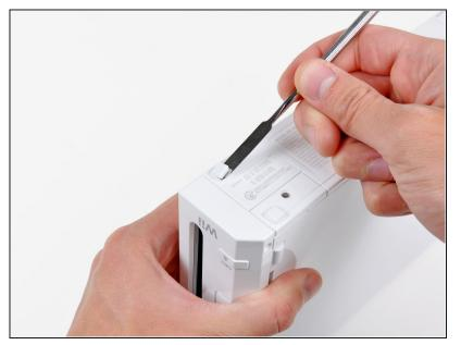
• Use a metal spudger to remove the rubber foot stuck to the side of the Wii near the DVD drive opening.
