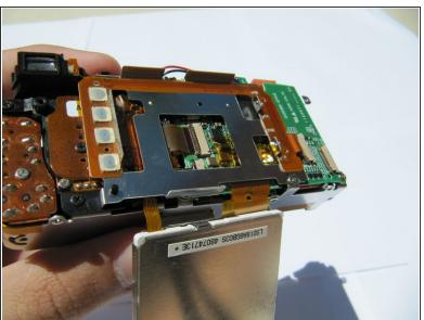
⚠ Carefully separate and flip over the LCD panel to expose the central circuit board.
