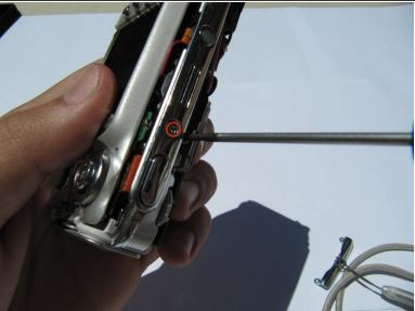
• Remove the top panel screw (1x 4.37mm).
