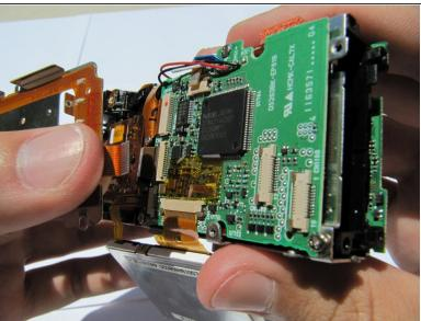
Pull the second orange tab from the circuit board and remove the buttons.
