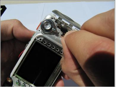
• Remove the back panel screws (1x 3.33mm, and 1x 3.40mm).
