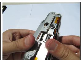
Separate the inner casing from the tripod mount.
