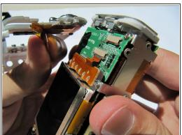
Gently pull the orange tab out of the circuit board.
