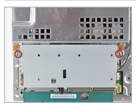
Remove the two 9 mm Phillips screws securing the memory card reader to the chassis.
