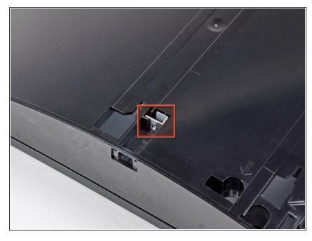
A Be sure to keep track of the small metal bracket loosely held in the top cover, if equipped.
