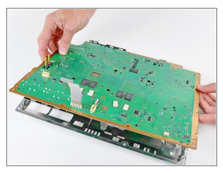
Remove the motherboard from the bottom motherboard cover.
