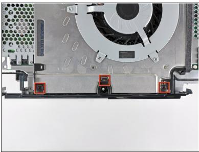
While lightly pulling the rear cover away from the logic board assembly, use the flat end of a spudger to release the clips along the top and bottom edges of the rear cover.
