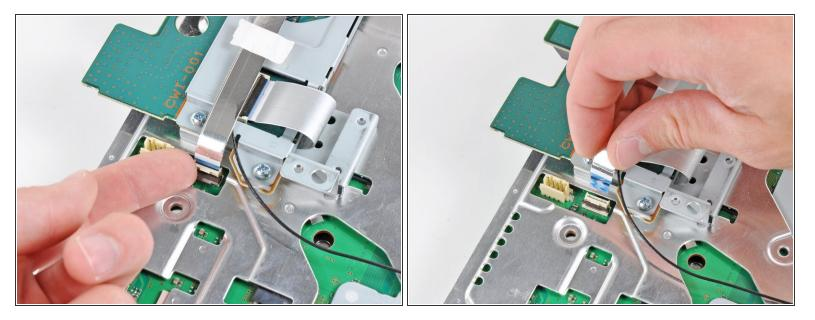
• Flip up the flap on the memory card reader ribbon cable socket and remove the ribbon cable.
