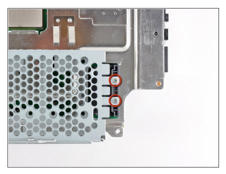
Remove the two 3.7 mm #0 Phillips screws securing the chassis to the hard drive socket.
