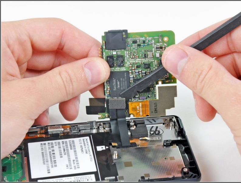
**i** Carefully lift the motherboard from the front case and lay it next to the Droid 2, minding the keypad connector that is still attached.
