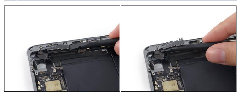
• Use the flat end of a spudger to cut the foam adhesive securing the antenna to the right speaker.
