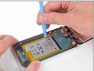
It took a bit of prying to lift the battery and logic board out of the casing, but unfortunately the headphone/sleep button control ribbon cable is both soldered to the logic board and glued to the outer case.
