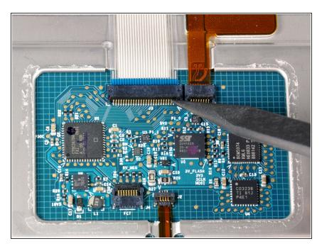
Use the tip of a spudger to flip up the black plastic flap locking down the orange upper case ribbon cable.
