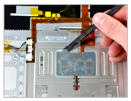
Use a spudger to pry up the translucent plastic sheet covering the keyboard connector. You can just peel up the three sides closest to the upper flex cable entering the keyboard connector to make it easier to reassemble it.
