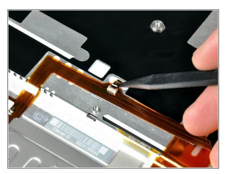
Use a spudger or your finger to slide the keyboard backlight ribbon out of its connector.
