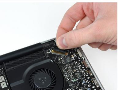
Grab the plastic pull tab secured to the display data cable lock and rotate it toward the DC-In side of the computer.
