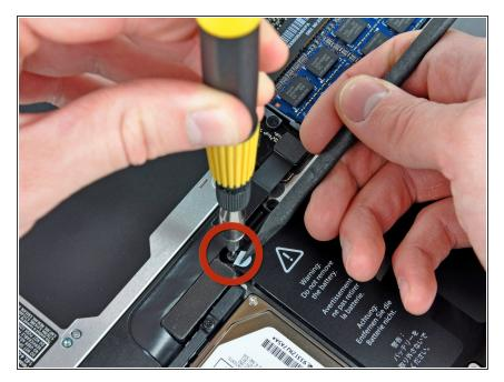
Use the tip of a spudger to bend back the finger of the "Warning: Do not remove the battery" sticker while you remove third five-point Pentalobe screw hidden underneath.
