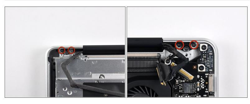
Remove the outer two T6 Torx screws securing both display hinges to the upper case (four screws total).
