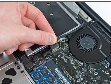
Pull the camera cable away from its socket on the logic board.
