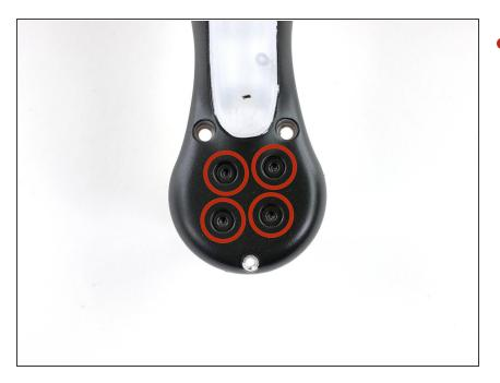
Remove the four 2mm hex motor bolts.
