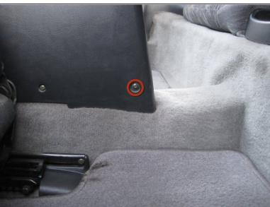
Remove the two Phillips screws at the very rear of the center console near the floor.
