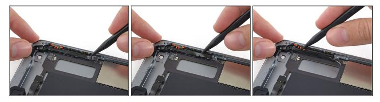
• Use the point of a spudger to separate the case button cable from the button cable mounting rail.
