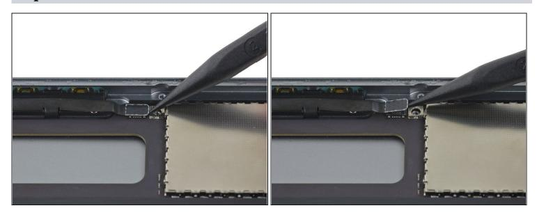
• Use the point of a spudger to lift the case button cable connector straight up out of its socket on the logic board.
