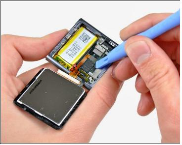
Use an opening tool to disconnect the display data and digitizer cable connectors up from their sockets on the logic board.
