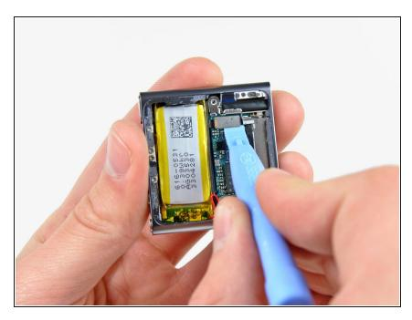
Use an iPod opening tool to lift the headphone jack assembly connector up and out of its socket on the logic board.
