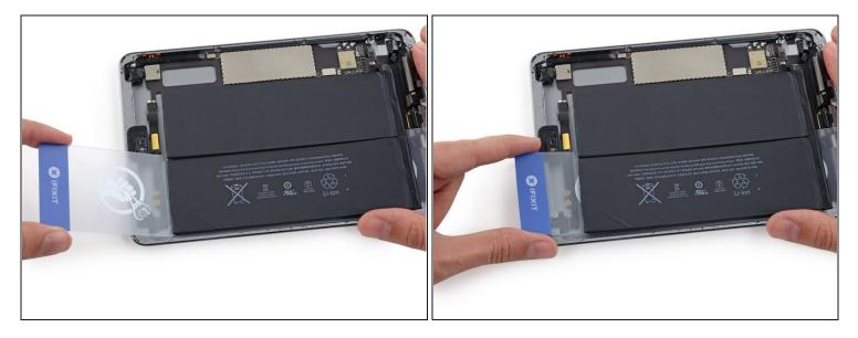
• Remove and insert the second card under the battery near the headphone jack.
