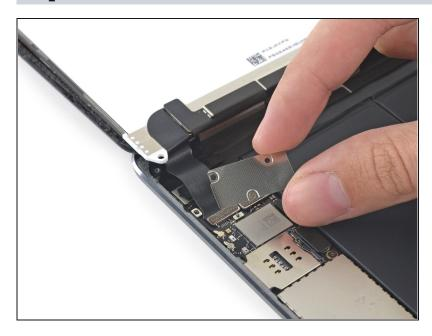
• Remove the display cable bracket from the iPad.
