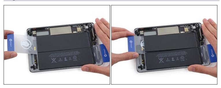
• Insert a second plastic card beneath the battery cell on the logic board side near the front-facing camera.
