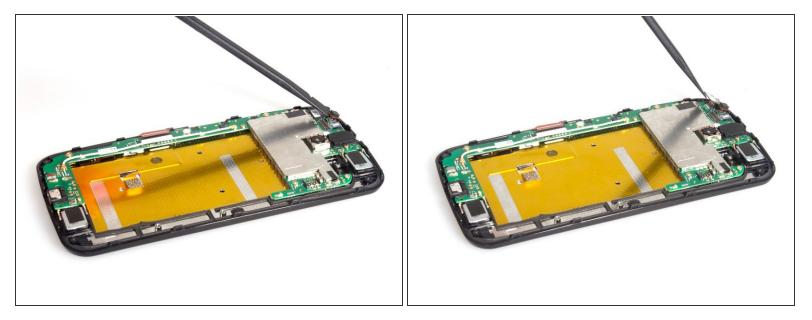
Release front camera connector and sensor connector.
