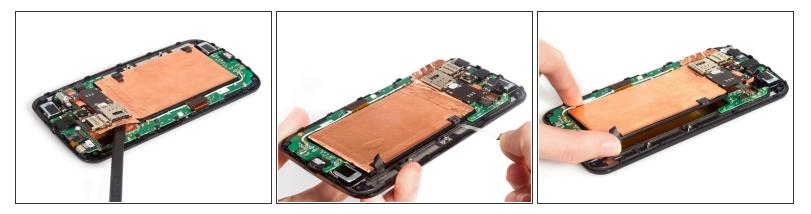
Loosen kinds of sticker under the battery and remove it with card reader assembly together.
