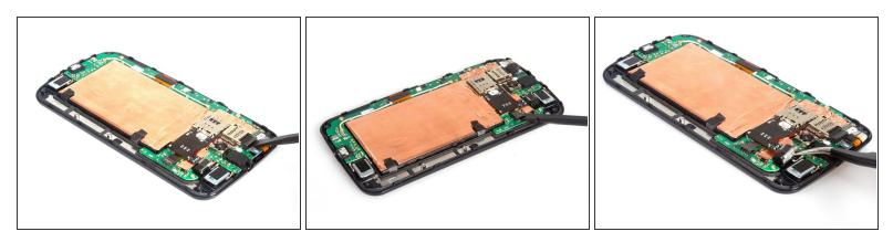
Release SIM&SD card reader assembly connector, battery connector and vibrator at first.
