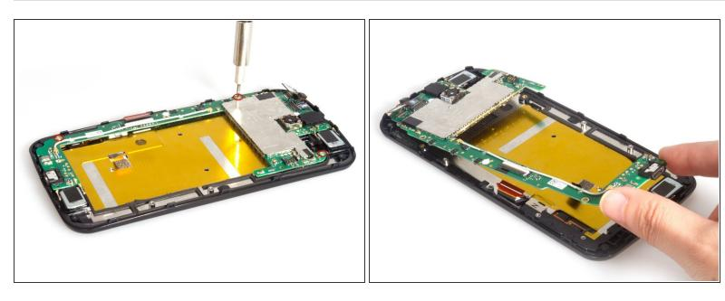
Remove three screws on the motherboard and take away the motherboard.
