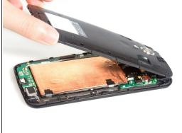
Remove back frame. The screws feature different sizes and lengths, so keep them in order after removing them.
