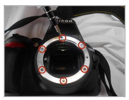
Remove the 6 Phillips screws on the front of the lens mounting ring.
