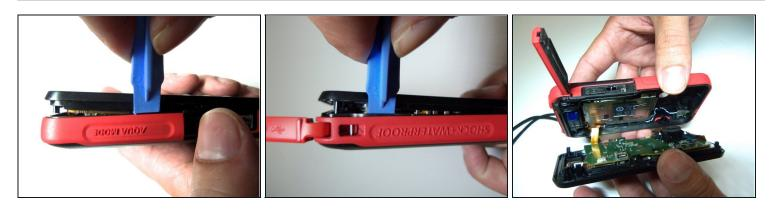
• Use the iFixit opening tool on both sides on the device. Pry apart both sections with light force.
