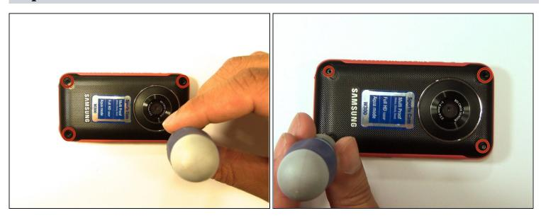
• Remove four screws with a Hex 1.5 mm screwdriver.
