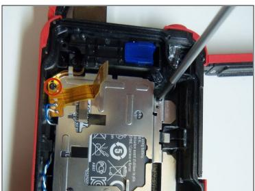
• Remove the four screws from the battery housing using a Phillips #00 screwdriver.
