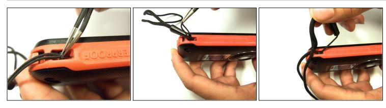
• To remove the wristband of the device, grab the middle loop and pull the band through.
