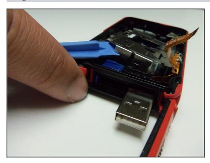
• Use the iFixit opening tool to pry the battery housing open.
