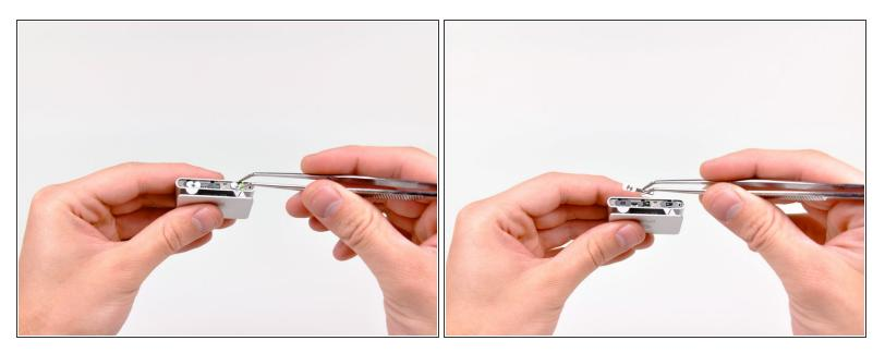
Use a pair of tweezers to remove the hold and shuffle sliders from the Shuffle.
