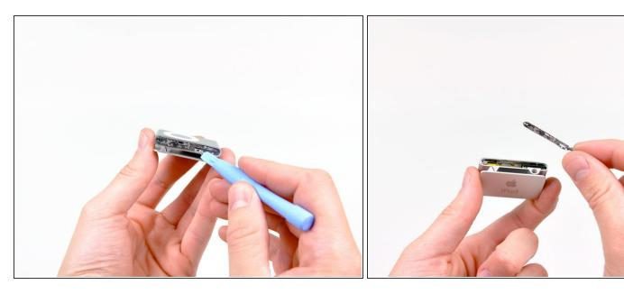
• Use the edge of an iPod opening tool to remove the steel cover from the headphone jack side of the Shuffle.
