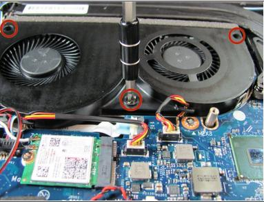
Remove the three 3.5 mm screws from the fan with a Philips #1 screwdriver.
