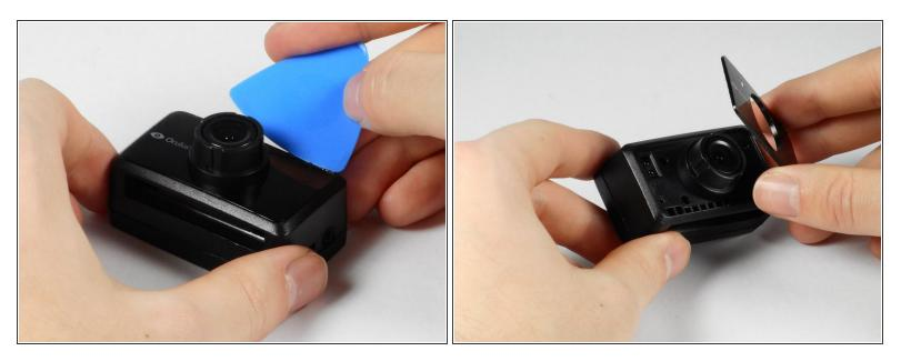
• Remove the cover plate from the front face of the camera using the iFixit Opening Pick.
