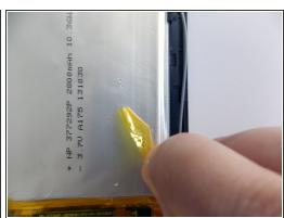
Remove the tape holding the battery in place.
